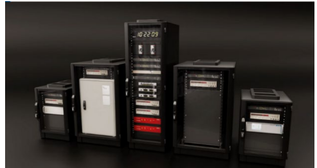
Fig. 1: 3D generated representation of one timescale composed of five racks. From left to right: OSA 3235B; iMaser3000; Control Unit; CSEM rubidium optical atomic clock; OSA 3300.
